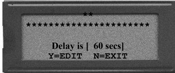
Press the 'Y' key to proceed in **EDIT**ing the current alarm delay or the 'N' key to return to Keypad options.
