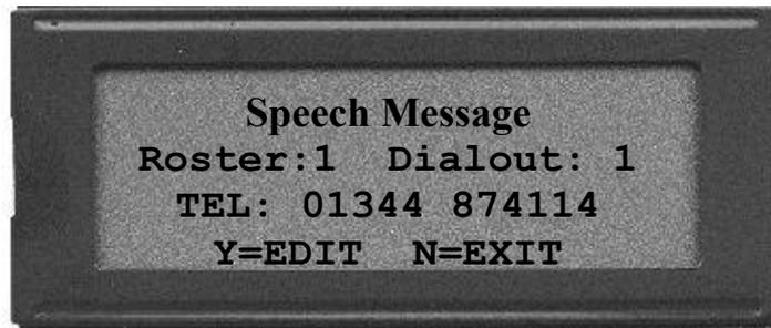
Line 1 'Speech Message', this is the type of call that will be made when you enter the telephone number. If the type of call you wish to make will be different to this (i.e. BT pager, Alpha pager etc), then press the 'M' key.
