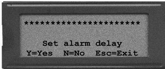
Press the 'Y' key to proceed in Editing the Alarm delay or the 'N' key to return to Keypad options.
